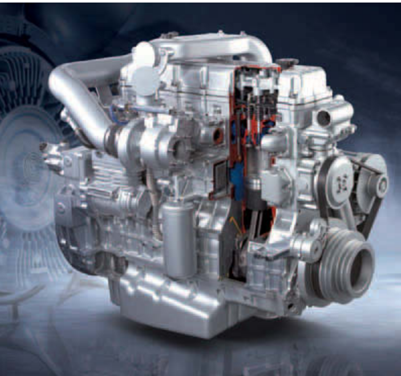
Motor “Common Rail” DLo8 de DOOSAN
