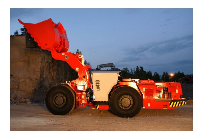
The Sandvik LH410 represents state of the art performance in difficult applications, enhanced operator ergonomics and several built-in safety features. High breakout forces, compact and lightweight unique design together with reliable structure ensures economical and reliable productivity. LH410 features a high lift boom enabling fast and accurate three-pass loading into the Sandvik TH430 truck.
