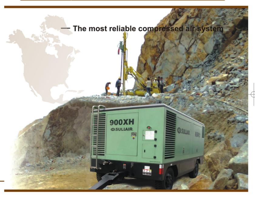
□ Driven by Cummins QSM11 electric injection diesel engine
